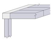
TYPE 3 Precast column and floor units with in-situ beams
