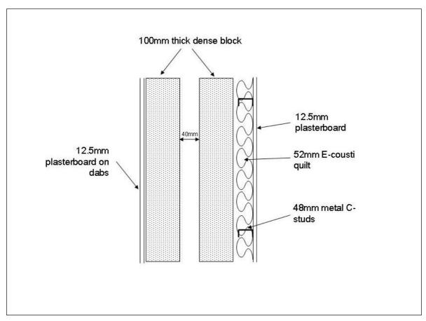
Figure 1: Separating wall construction between adjacent dwellings at 115 Llandudno Road, Colwyn Bay
