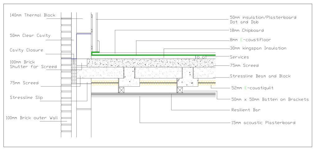
Figure 2: Separating floor construction between adjacent dwellings at 115 Llandudno Road, Colwyn Bay
