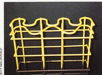
There have been successful trials of coating complete fabricated cages by fluidized bed dipping.
