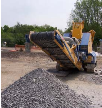
An in-situ crusher producing CCA (From NF45 The use of recycled materials in residential NHBC Foundation)
