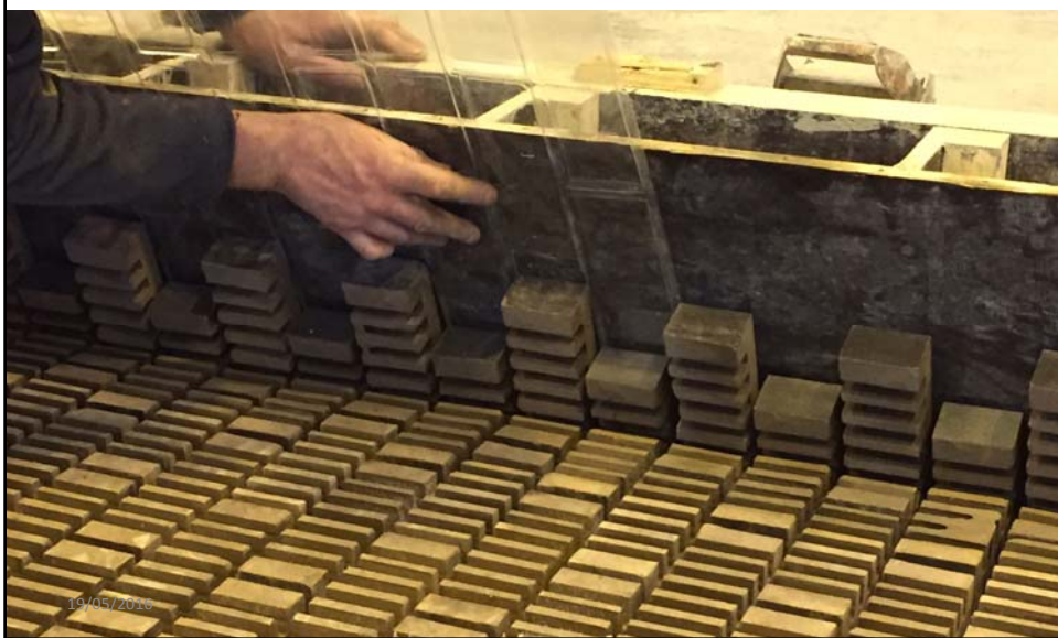
Cut brick set out in the mould
