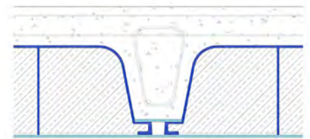
2 Cross-section of detail with GRP void former and ply insert covering joints between trough sections
